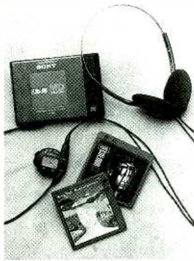
FIG. 1. SONY'S MINIDISC (MD) digital audio format uses ATAC digital data reduction compression to fit the same amount of music on a 2.5-inch disc as is found on full-size compact discs.
